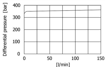
Flushing valve characteristic
