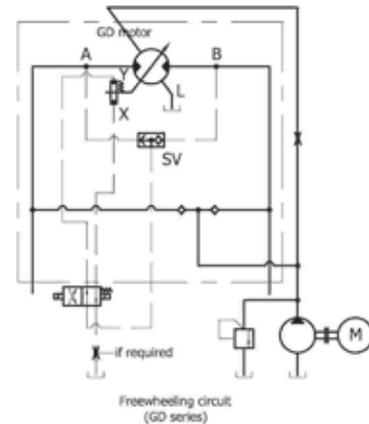
Selecting a G series hydraulic motor, the following circuit represents the best choice for freewheeling operation. The motor works under vacuum conditions, therefore it can work several hours without causing any damage and overheating. The switch from normal operation (and viceversa) must be done at low speed and pressure. Consult Italgrou technical department to obtain more details.
