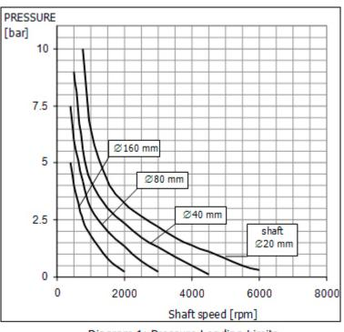
Diagram 1: Pressure Loading Limits
